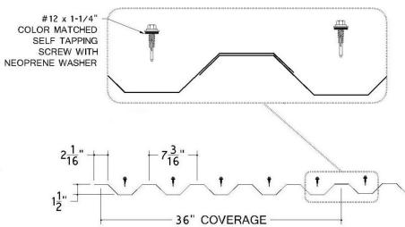
Economical and structural, the 7.2 steel wall panel is a versatile, exposed-fastener design that compliments a variety of buildings types.
