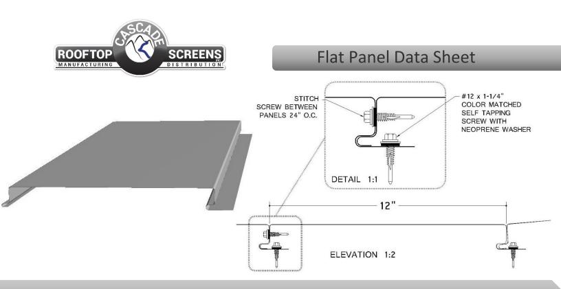
Flat and flush, this steel panel creates a wall that has no bumps or ribs. Used when you have a screen that needs to blend in with surrounding walls.
